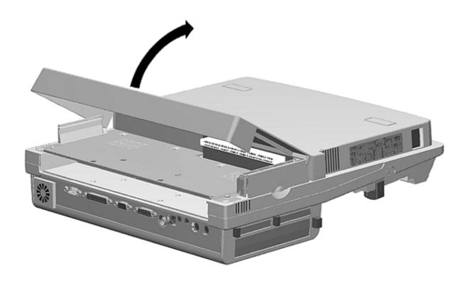
Figure 7-10. Removing the ISA Cover Assembly
